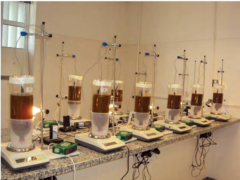
Figure 1. Nine fermentation tanks equally distributed on three temperatures (30 °C, 33 °C and 36 °C) with individual temperature controllers.
