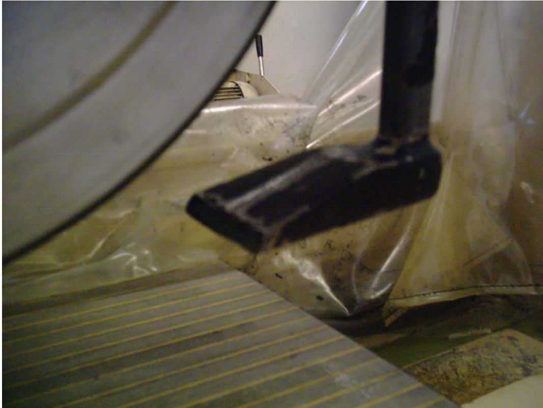
Figure 1. Picture of grinding through lubrication-cooling with conventional nozzle.
