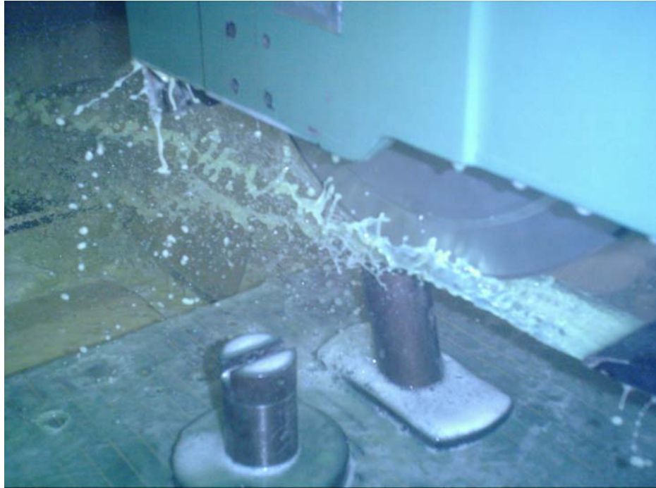
Figure 5. Grinding wheel profiling operation.
