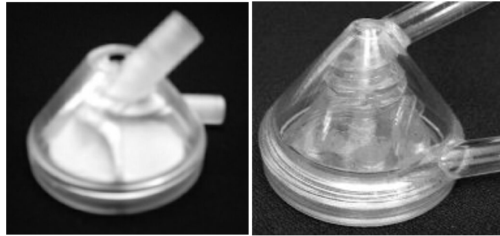
Figure 4. Pump one with inlet port angle of 30° and pump two with inlet port angle of 45°.
