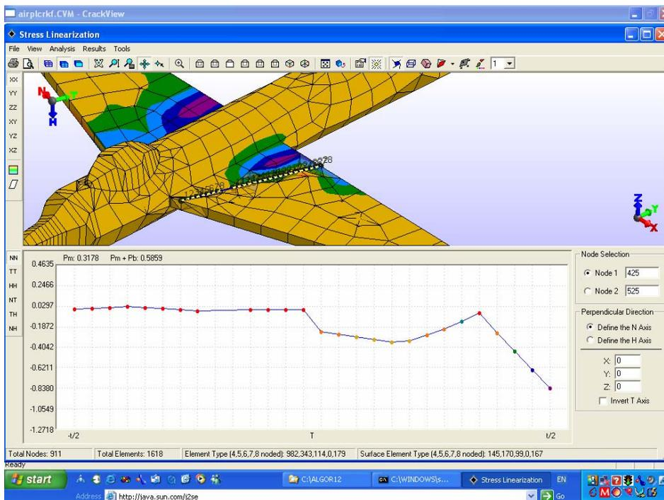
Figure 5. Stress linearization shown via Crackview's CAE module integrated with ALGOR commercial software.
