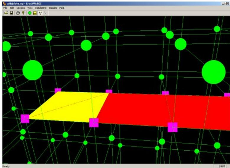
Figure 6. Insertion of an user-defined crack (red and yellow color) at node level
