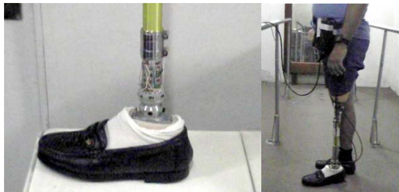
Figure 5. Three-axial transducer in the amputee.
