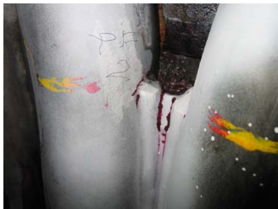
Figure 8. Crack at the lower crotch plate of primary air ports
