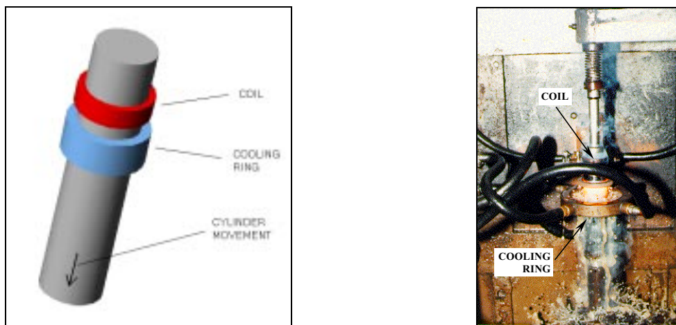
Figure 1. Experimental apparatus for progressive induction hardening.
