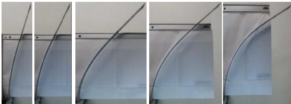
Figure 3. Buckled column. Deformed shapes for increasing length.
