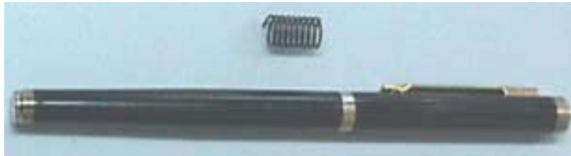
Figure 3 – Picture of the SMA coil spring obtained by the thermomechanical procedure indicated in figure 2.
