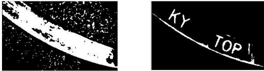
Figure 3. Left: the first threshold and grouping operations, to find out the ring; Right: the second threshold and grouping operations, to find out the characters.
