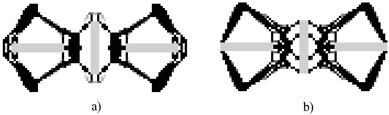
Figure 8: Topology optimization result: a) w equal to 0.9, \alpha equal to 0.3, and \beta equal to 0.7; b) w equal to 0.8, \alpha equal to 0.8, and \beta equal to 0.2.
