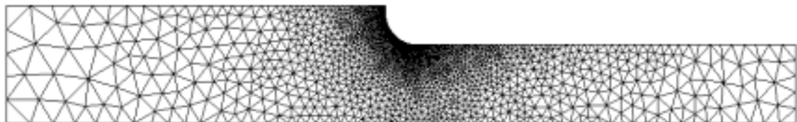
Figure 5. Typical finite element mesh, r/d = 0.2 , D/d = 1.5 .
