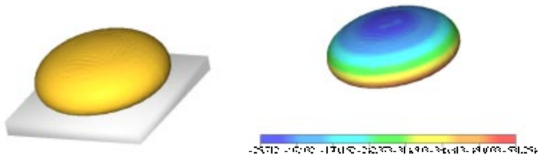
Figure 10. Volume rendering with Phong shading (left) and pressure using pseudo-colors (right) of a sessile drop. Steady state ( t = 1.0 ), B_o = \rho g D^2 / \sigma = 7.884 , dx = dy = dz = 0.05D , where D is the bubble diameter.
