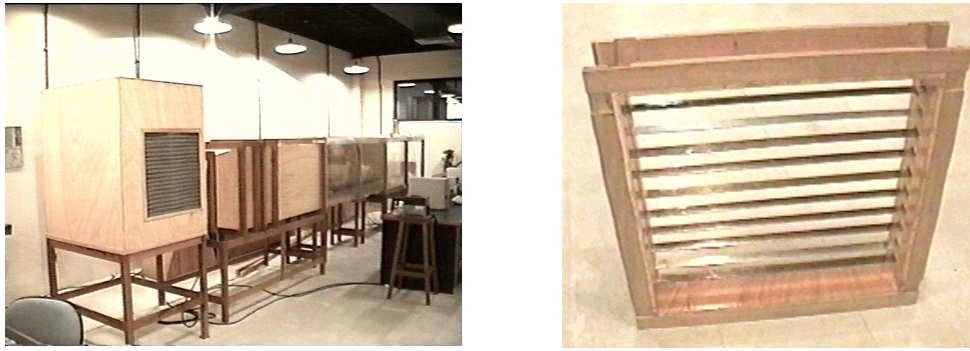
Figure 1. Wind tunnel configuration with heating rods detail (right).
