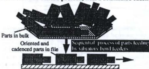
Figure 1: The parts feeding problem by vibratory bowl feeders.
