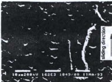
Figure 7: The worn surface of Thordon XL in dry sliding versus plasma-sprayed  $\text{Al}_2\text{O}_3$  coating under 45.3 N normal load at a speed of 1 m/s.
