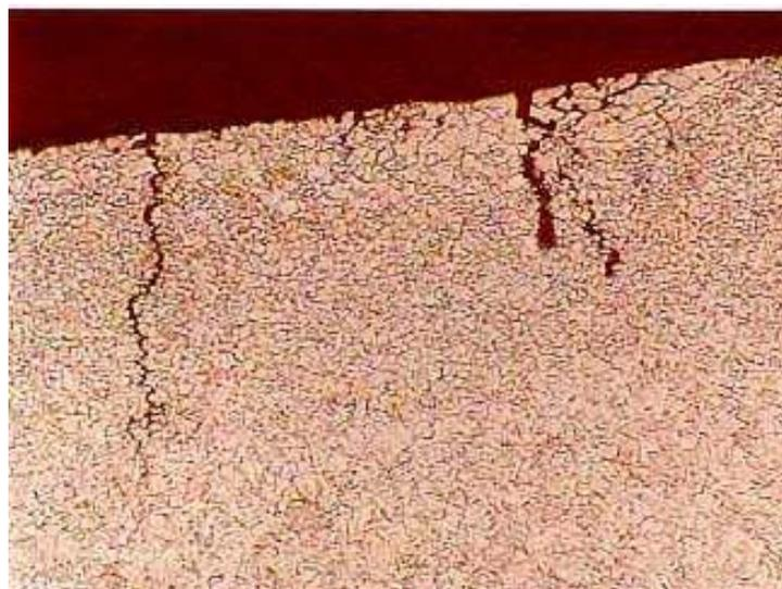
Illustration 13. Micro cracks found in a burnt spot (100X).
