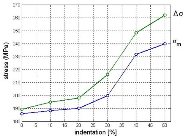
Illustration 16. Maximum main stress components variation in function of spotweld indentation. Results of the simulation through FEM with solid elements.
