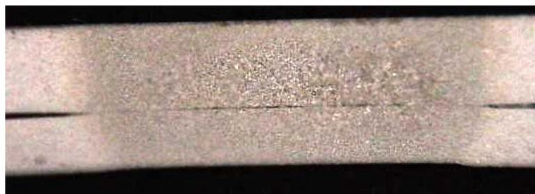
Illustration 6. Macrograph of a cross-sectioned stick weld
