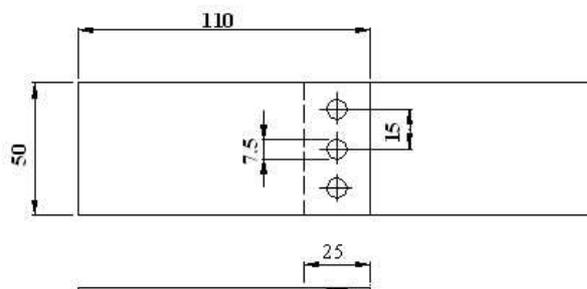
Illustration 1. Welded specimen in study and spot weld geometry.
