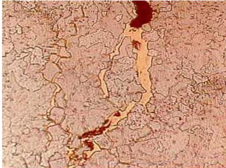
Illustration 14. Micrograph of a burnt spot, showing a copper deposit inside the micro crack (200 X).
