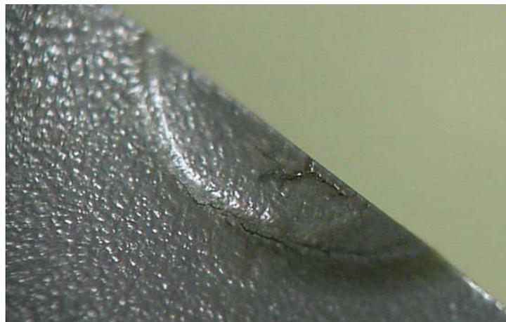
Illustration 12. Macrograph of a cross-sectioned burnt spot.
