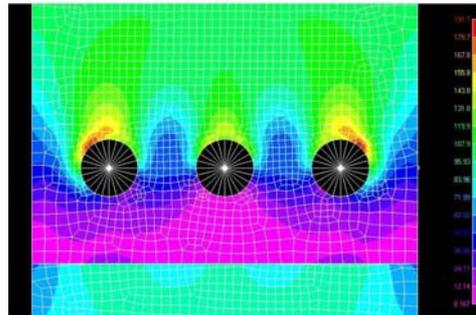
Illustration 15. Results of the simulation through FEM for the von Mises stress with plate elements, showing area of  $\sigma_{med}$  concentration in the most external spots.
