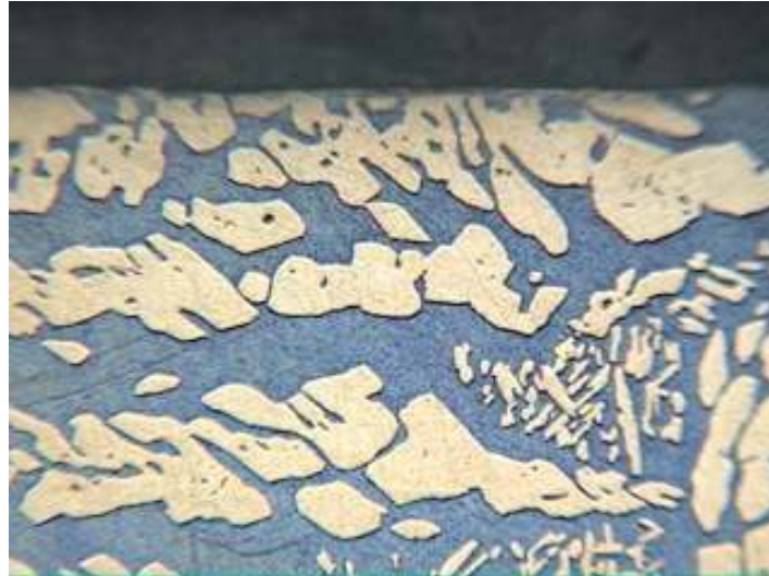
Figure 4. Optical analysis of a specimen (Cutting speed = 80 m/min; feed rate = 0.25 mm/r; cutting depth = 2 mm; with cutting fluid; carbide insert class 2015) etched by modified Behara
