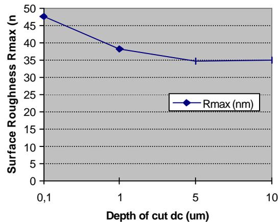
**Figure 3.**  $R_{max}$  value as function of depth of cut.
