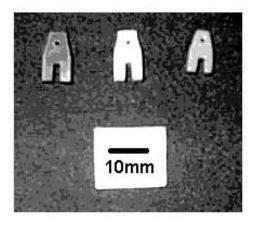
Figure 4 – Granite thread-guides
