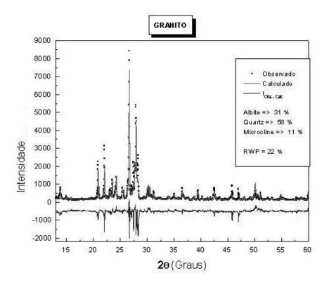
Figure 1- Diffractogram of "Asa Branca" Granite
